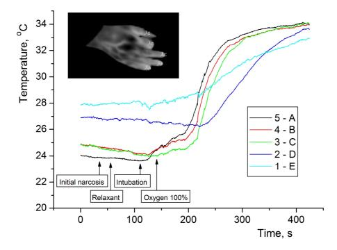
**Fig. 6.** Temperature change of fingers of the patient's right arm on a surgical table during premedication and initial narcosis. Checkpoints A, B and C are situated in and around the nail bed of the fifth, fourth and third fingers, point D and E – on the phalanges of the second and first fingers, respectively.
