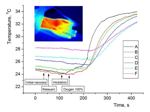
**Fig. 7.** Time profiles of the temperature measured in several points along the patient's fourth finger on the stage of premedication and initial narcosis before surgical operation. Checkpoints A–F are located proximally starting from the nail bed.
