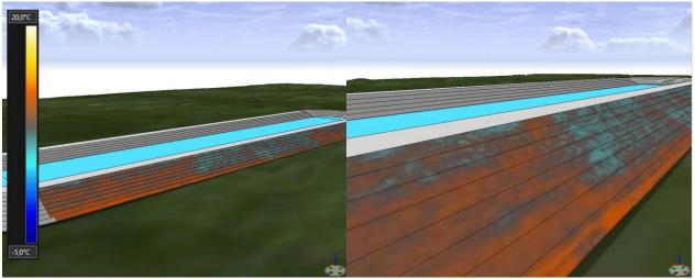
Fig. 1. 3D GIS model of experimental embankment using infrared images.
