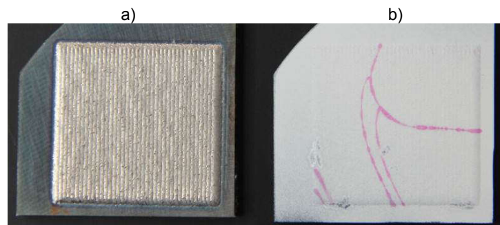
Fig. 3. Laser deposited coatings: before (a) and after PT test (b)
