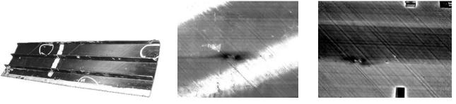
Fig. 4. Curved CFRP landing flap. Photograph (left), Halogen lamp (center) and VCSEL (right) excited lock-in thermography results.
