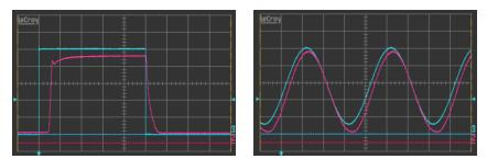
Fig. 7. Left: Delay of output current pulse with maximum control input overdrive. Output current (magenta) and analog control signal (cyan). Timebase 2 ms/div. Right: 50 Hz sine modulation. Output current (magenta and analog control signal (cyan). Timebase 5 ms/div
