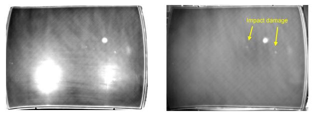
Fig. 5. Halogen lamp (left) and VCSEL (right) excited lock-in thermography results for the large CFRP part
