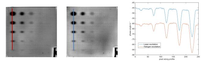
Fig. 2. FBH specimen tested at 0.095 Hz lock-in-frequency with Halogen lamps (left) and VCSEL (right). Comparison of phase profiles on the right.
