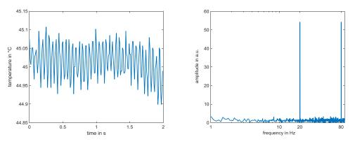
Fig. 8. 20 Hz thermal signal from the specimen surface recorded with IR camera (left) and Fourier analysis thereof (right)
