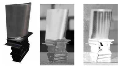
Fig. 6. Titanium turbine blade: Photograph (left), Halogen lamp excited lock-in thermography result (center) and VCSEL excited lock-in thermography result (right)
