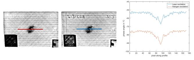
Fig. 3. CFRP Impact specimen tested at 0.25 Hz lock-in-frequency with lamps (left and VCSEL (center). Comparison of phase profiles on the right.
