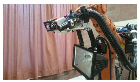
**Fig. 2.** Three-dimensional thermal imaging system existing of a MESA SR4000 time-of-flight camera (left), a XENICS Gobi 640 thermal camera (middle), a CMOS uEye UI124xSE RGB camera and a 500 Watt halogen light.
