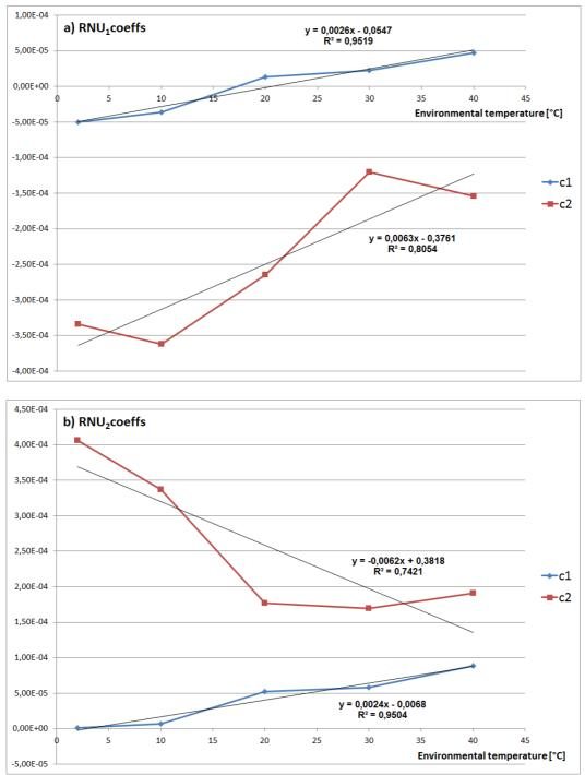
Fig. 3. Graphs of c1 and c2 coefficient changes in function of the temperature of climatic chamber and their approximation with the linear function
