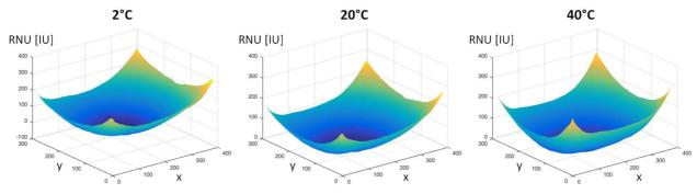
Fig. 2. 3D visualisation of RNU characteristics for different temperature conditions of working camera
