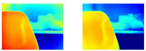
Fig. 5. . False color images of office interior before and after developed RNU correction
