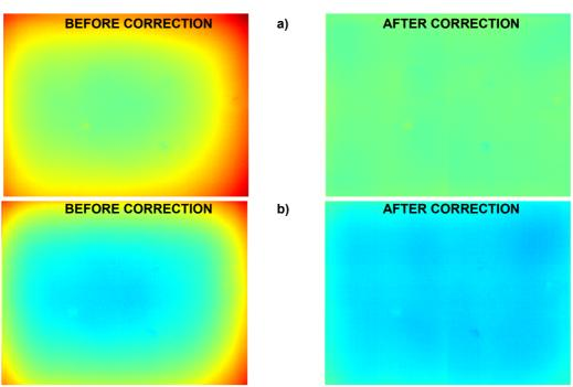
*Fig. 4.* False color images of black body (set to 40°C) before and after developed RNU correction for two different temperatures of camera working environment. a)  $T_{ambient}$ =20°C b)  $T_{ambient}$ =40°C
