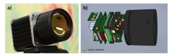
Fig. 1. The designed infrared camera (a) and its perspective view of interior with marked sensors positions (b)
