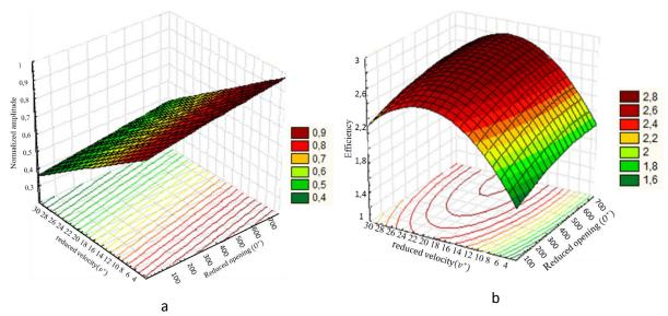
Fig 7 : Influence of travel velocity and opening on bipolar amplitude signal, a: normalized amplitude, b: efficiency
