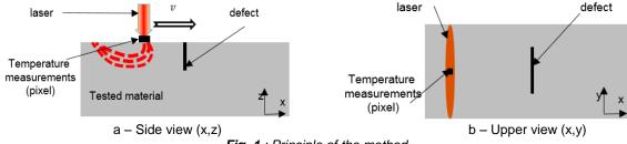
Fig. 1 : Principle of the method
