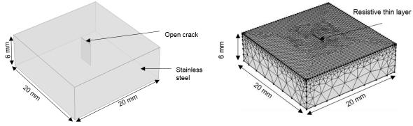
Fig 4 : Geometry and meshing of the examined material
