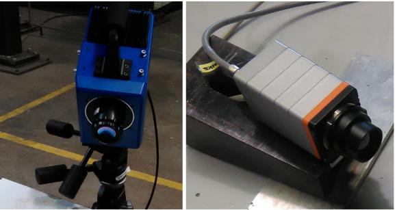
Fig. 3: Thermal cameras for the induction thermography study: FLIR SC7600 (left), Gobi 640GigE from Xenics (right).
