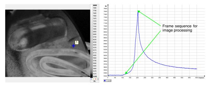
Fig. 4: Example of time evolution for a given pixel in the induction area next to the coil.
