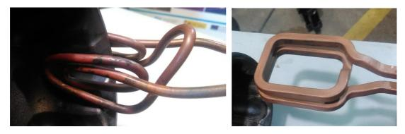
Fig. 7: Internal coil for both transversal and longitudinal (left) and external coil for longitudinal crack detection (right).
