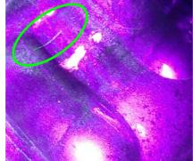
Fig. 1: Steel part under magnetic particle inspection. The crack is indicated with a green marker.
