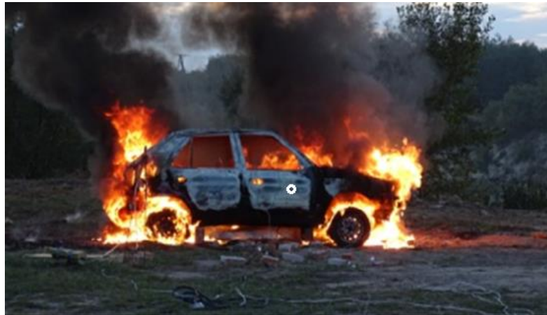
Fig. 6. The car in the final phase of burning. The measurement area is marked by a circle on the car body
