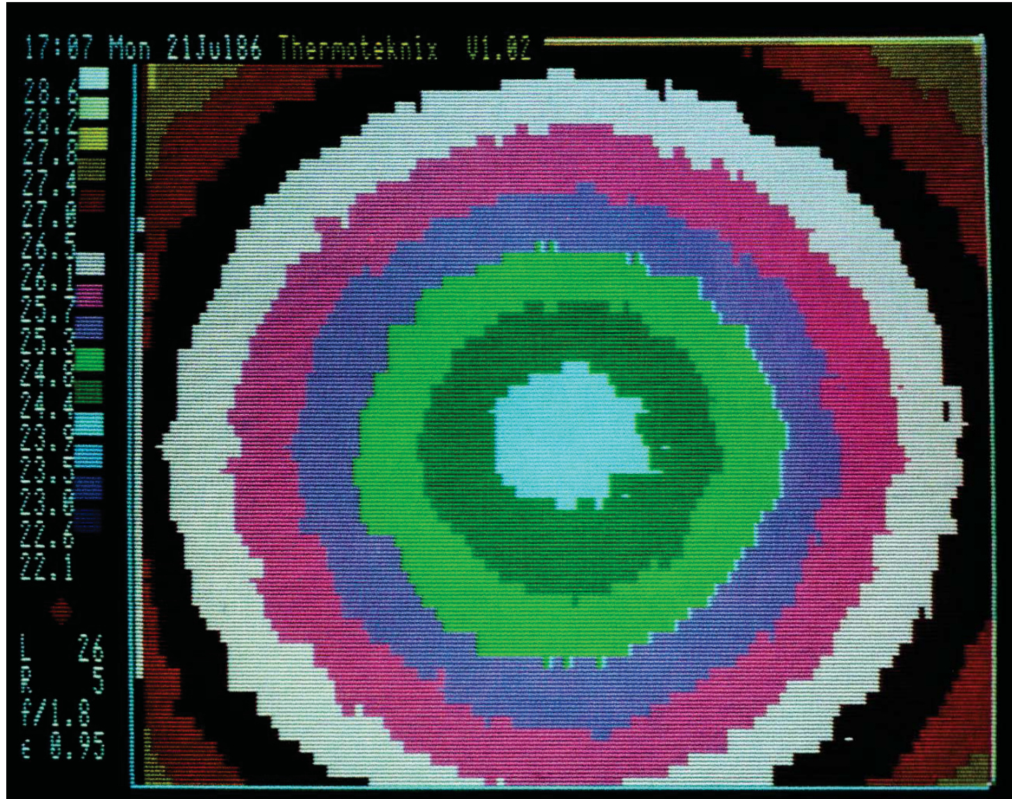
Jet impinging on a plate, contours of constant temperature; z/d=6 , Re=28000 (1986). To my knowledge, shows the first thermographic image of an impinging jet.
