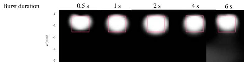
**Fig. 2** Gray level representation of the heat source distribution obtained from experimental data corresponding to calibrated homogeneous heat sources (delimited by the red contours), for different burst durations. White represents maximum value of the retrieved heat flux and black is absence of heat sources.
