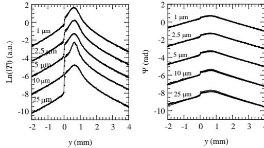
**Fig. 1** Experimental surface temperature profiles (symbols) perpendicular to infinite calibrated cracks, through the center of the laser spot, and fittings to the analytical model (continuous lines).
