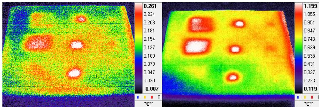
**Fig. 2** Thermograms of the concrete sample at  $t = 100$  sec for heating time of 25 sec and 100 sec.
