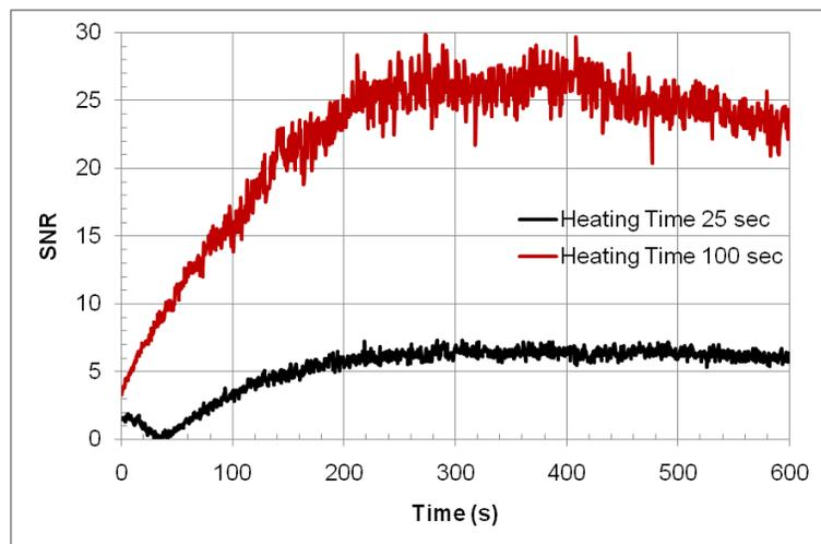
**Fig. 3** SNR variation as a function of time for defect of size 10 cm x 10 cm at 1 cm depth.
