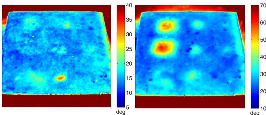
**Fig. 1** Phase images of concrete sample at  $f = 0.005$  Hz and 0.001 Hz.
