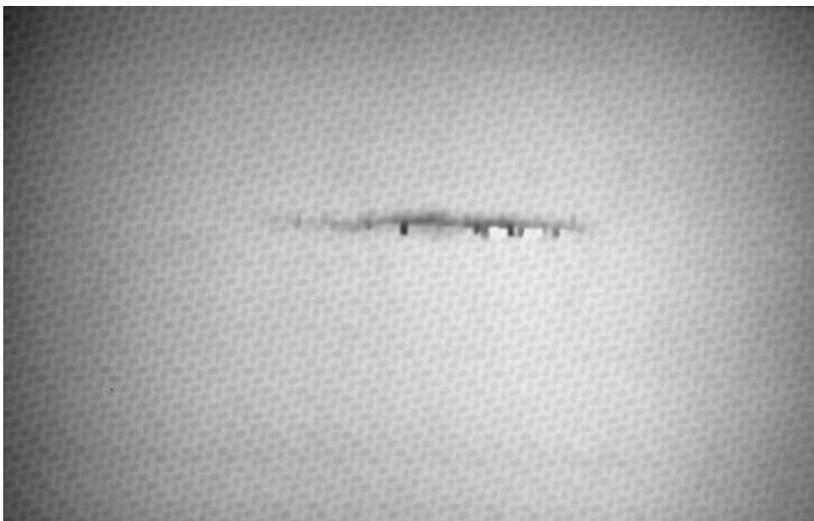
**Fig. 2** Thermogram of single plate after shoot lead projectile (transmission approach).
