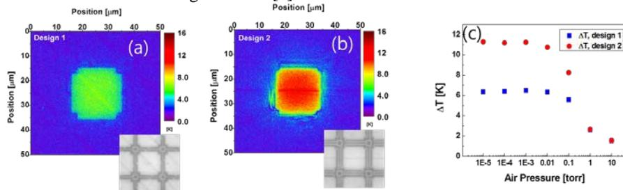
Fig. 3. Thermal distribution images of microbolometer (a) design1 and (b) design2 measured by TRM system at 1 V bias. (c) Average temperature variation of microbolometer design1 and design 2 as a function of pressure in vacuum package
