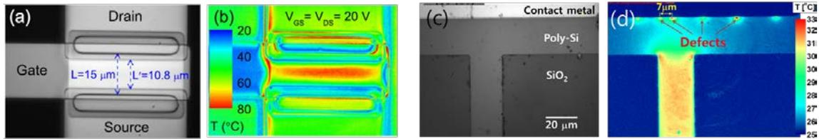
Fig.2. IGZO short channel TFT (a) Optical microscope image (b) Temperature image; Poly-Si micro-resistor (c) Optical microscope image (d) Temperature image
