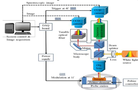
Fig. 1. Schematic of a thermoreflectance microscope system
