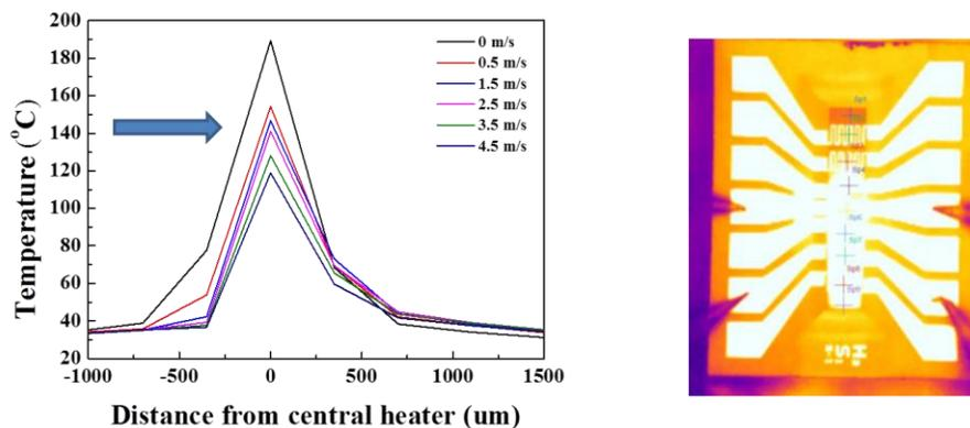
Fig.2 The temperature changes of flow sensor and infrared image according to the flow rate.
