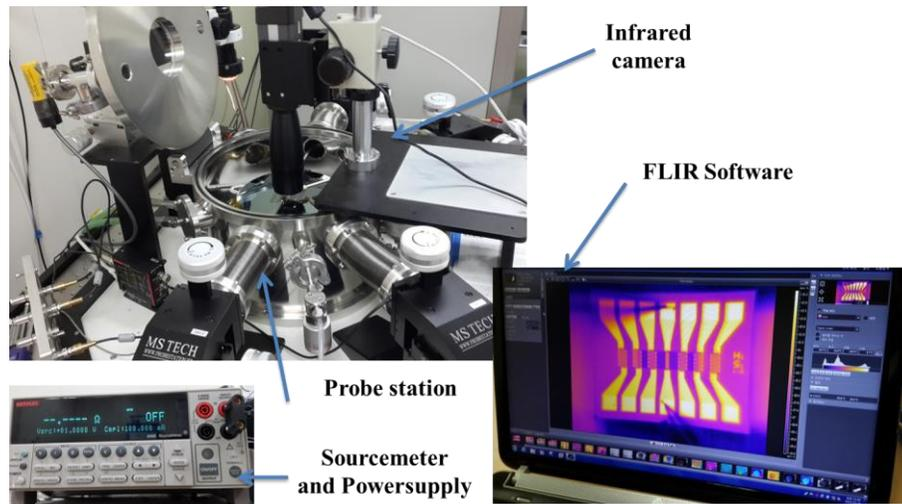
Fig. 1 The measurement setup.
