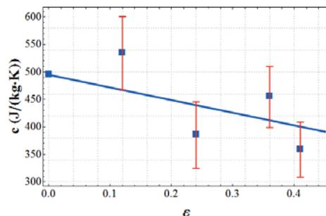
Fig. 1 A dependence of the heat capacity of the stainless steel AISI 304 on the deformation.
