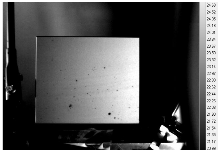
Fig. 3 Thermography of FTO thin film with the defect due to impurities.
