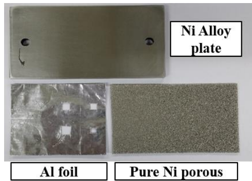
Fig. 4 Components of the porous/bulk titanium bonding composite with artificial defects made by perforated filler metal.
