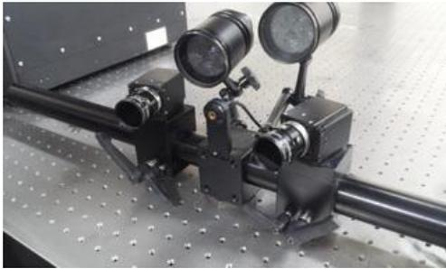
**Fig. 2** Experimental DIC setup using stereo vision for measuring tensile stress on the standard tensile specimen.
