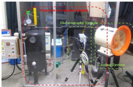
**Fig. 7** Experimental Shearography setup for detecting inner defect of a pipe in heating circulation system.
