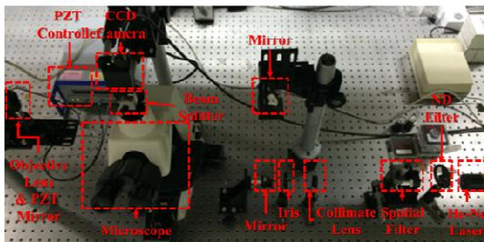
**Fig. 4** Reflection type digital holography setup.
