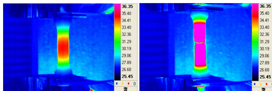
Fig. 1 The entire thermographic images of axle material in diesel electric locomotive during tensile testing.
