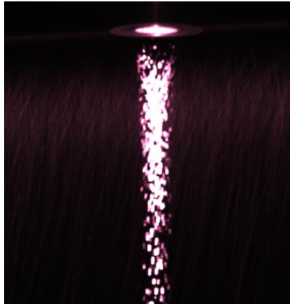
Fig. 4. Image of laser beam scattering on powder particles obtained with VIS/NIR Mako G-125 camera (II-a)
