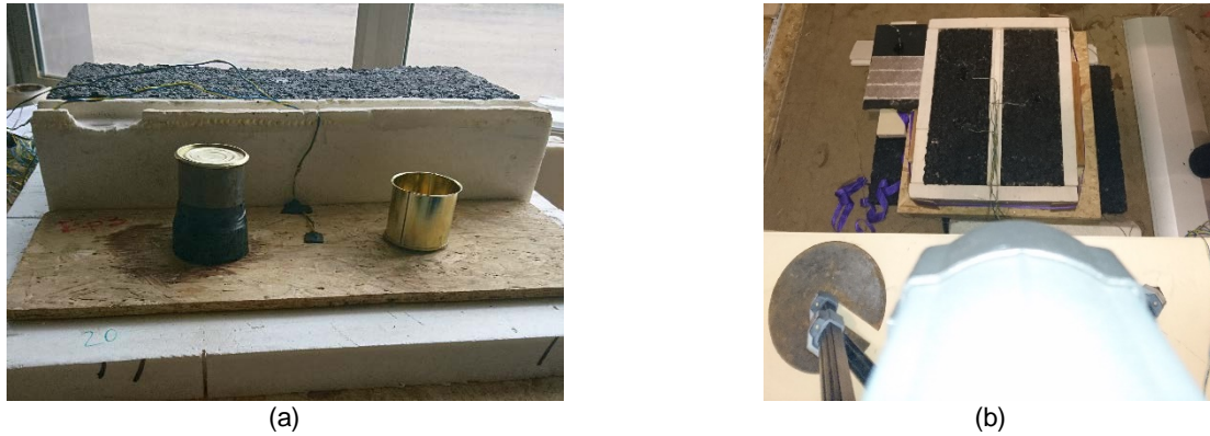
Fig. 1. Pristine pavement sample and PCM metallic containers before installation of pavement sample with voids with T-type thermocouples (a) and pavements samples with FLIR A320G infrared camera (b)
