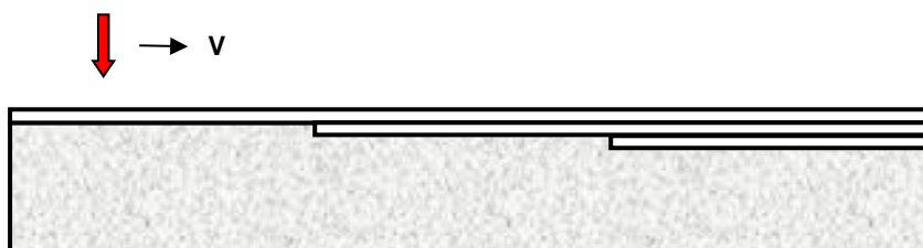
Fig. 2. Model of a metal sample covered with paint layers
