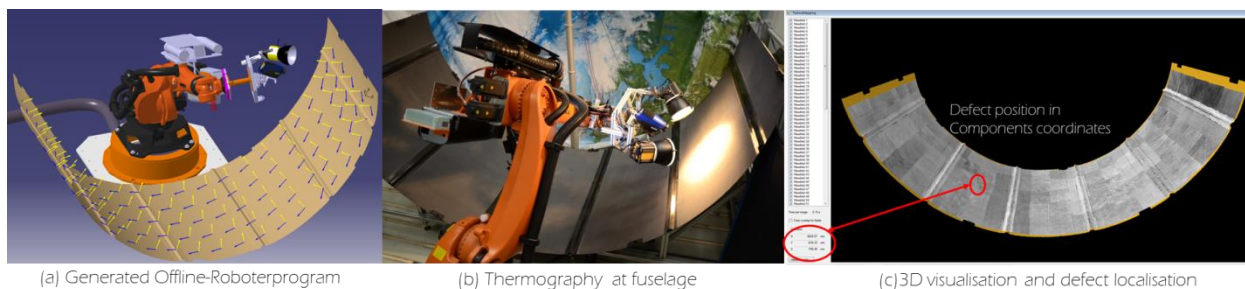
Figure 10: (a) generated offline-Program; (b) Experimental setup; (c) 3D visualisation and defect detection
