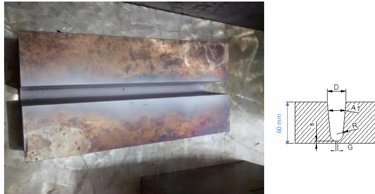
Fig. 1b: Characteristics of TIG multipass narrow gap welding.
