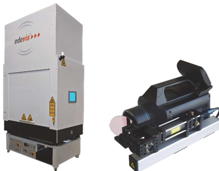
Fig. 3: Industrialized laser cabin (left) and Forakam demonstrator based on FLIR X6580sc (right).
