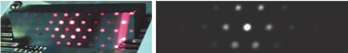
Fig. 6: Multispot laser excitation by a diffractive optical element (left), amplitude image showing the different energy density of the laser spots (right).
