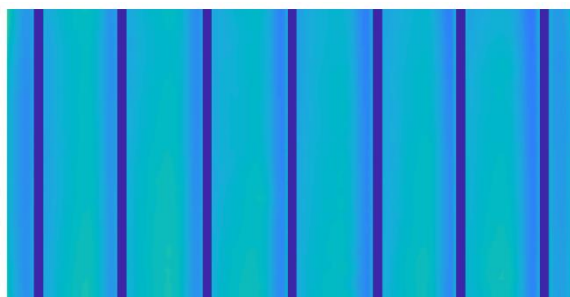
Fig. 14: Heat transfer coefficient distribution for p/e = 10 and e/\delta = 0.4 .
