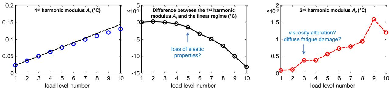
**Fig. 2:** Variations of the first and second harmonic moduli during a self-heating test from one load level to another (left & right). Highlight of the nonlinearity of the first harmonic (middle).
