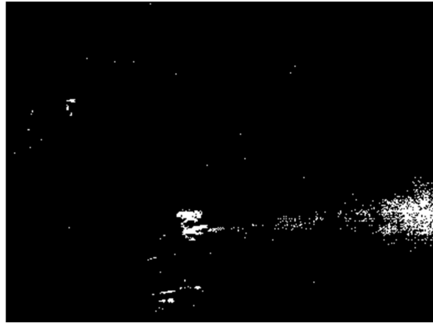
Fig. 9: Segmented image after background removing from the sequence of thermal images during the propane-butane leakage
