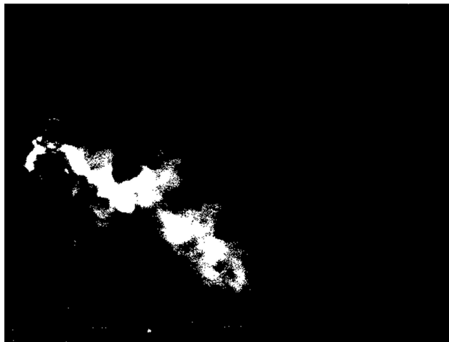
Fig. 6: Segmented image after background removal from the sequence of thermal images during monitoring the ammonia leakage
