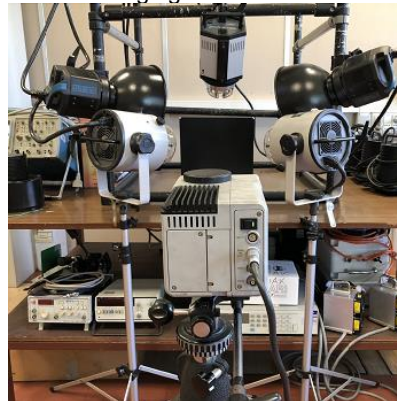
Fig. 1. Experimental layout. The thermal camera is pointed at the specimen which is thermally stimulated by a set of lamps.
