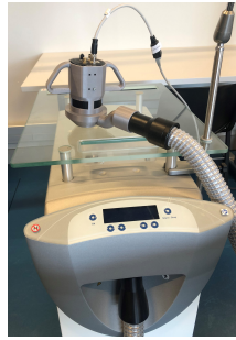
(a) Cryo cooling unit and measurement head
