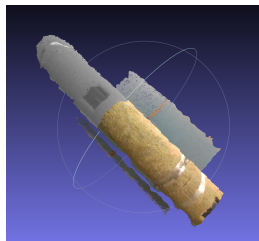
Fig. 1. Sample point cloud collected by the platform from an insulated pipeline under laboratory conditions. The figure shows the point cloud with thermal and visible values.
