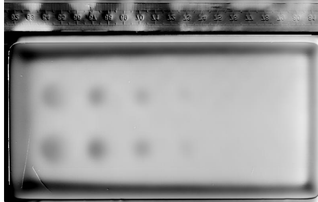
Fig.3. Phase image of a steel workpiece with flat bottom holes obtained from a manual scan; flat bottom holes in upper row with 8 mm diameter; flat bottom holes in lower row with 10 mm diameter
