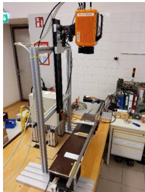
Fig.1. a.) Test rig for scanning with an inductive linear heating source; b.) Test rig for scanning with a U-shaped inductor
