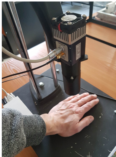
Fig. 3. Measurement stand with IR cooled single-detector head
