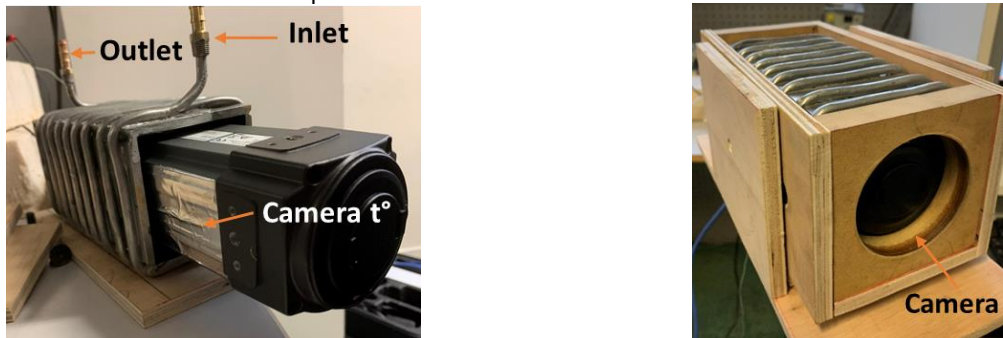
Fig. 2. Cold box with cold water circulation (fig. 2a) for the FLIR A325sc thermal camera (fig2b)
