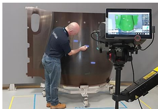
Fig. 10. Thanks to digital thread, indications identified with Flash Thermography are located on the part with augmented reality device
