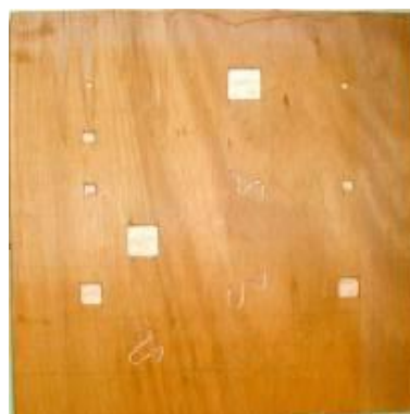
Fig. 1. Defects machined inside the support structure of the studied chessboard
