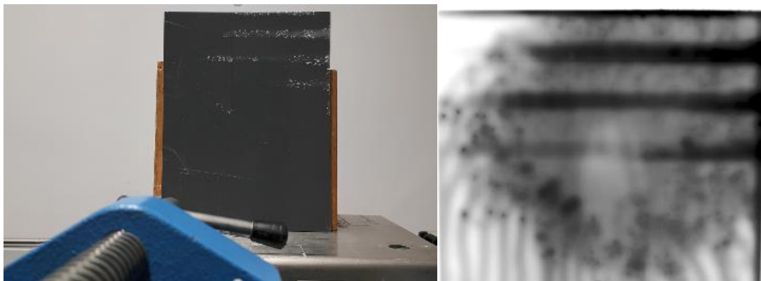
c) Sublimation of the frost layer, left: visual image, right: infrared image
