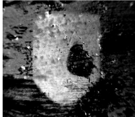
Fig. 8. Pulsed thermography shows the decal. The paint is not transparent in the IR and nothing is visible except the shape of the decal.
