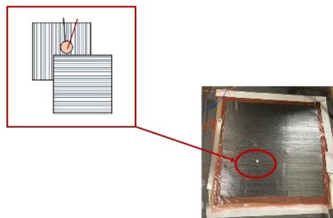
Fig. 1. Schematic representation of the PZT located between two plies of a T700-M21 laminate composite [2]
