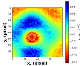
Fig. 2 Velocity map resulting from the Lamb waves generated by the embedded piezoelectric transducer into composite plate.
