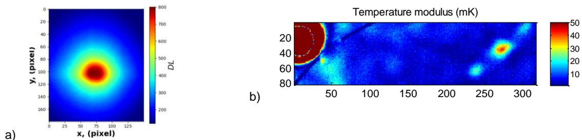
Fig. 4. a) Heat diffusion from the PZT transducer embedded inside a composite plate and b) detection of an impact damage in the laminate composite, by lock-in thermography. The PZT transducer is attached to the surface of the coupon.
