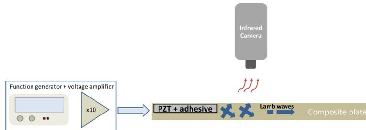
Fig. 3 Vibrothermography bench used to image the thermal response of a defect revealed by Lamb waves excited by a PZT transducer embedded inside a composite plate.
