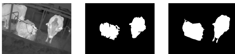
Fig. 3. Association of both DenseCRF and the Fast Bilateral Solver to the segmentation of animals. From left to right, original image, refinement of the raw segmentation mask using DenseCRF, improvement of the output of the DenseCRF algorithm using the Fast Bilateral Solver.
