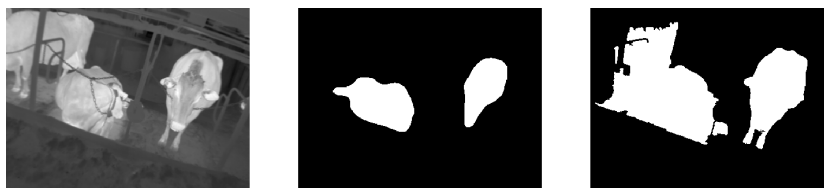
Fig. 2. Application of the Fast Bilateral Solver to the segmentation of animals. From left to right, the original image, the segmentation mask refine, the segmentation mask raw.
