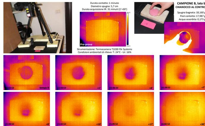
**Fig. 1.** IR camera looking at the process of evaporation after the contact sponge application (top left). Application of the contact sponge (top right). Some IR images showing the evolution of the evaporation and diffusion of water in the porous material (middle and bottom rows).
