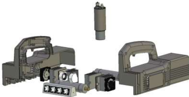
b) thermal NDT scanning device (details)
