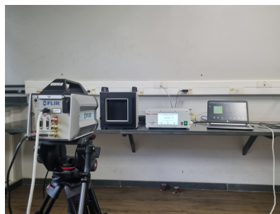
Fig. 4. Calibration setup for the MWIR camera equipped with a spectral filter.
