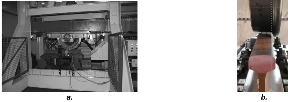
Figure 6. a. Image of the full-scale rail wheel test rig published in [12]; b. initial position of the wheel over the rail
