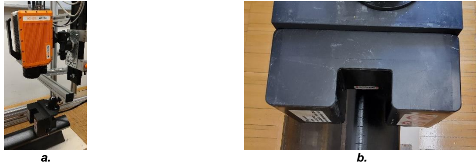
Figure 9. a. Laboratory setup for static inductive measurements on a rail head; b. Close-up of the inductor
