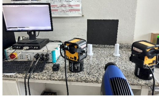
Fig. 3. Photograph of the experimental setup used to carried out the PT and PPT tests.
