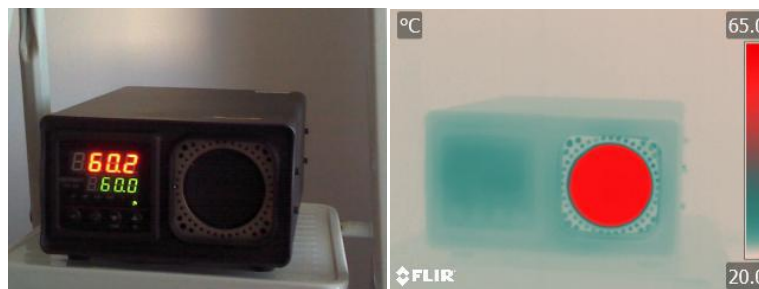
Fig. 1. Thermogram isothermal surface of the IRS-350 black body.
