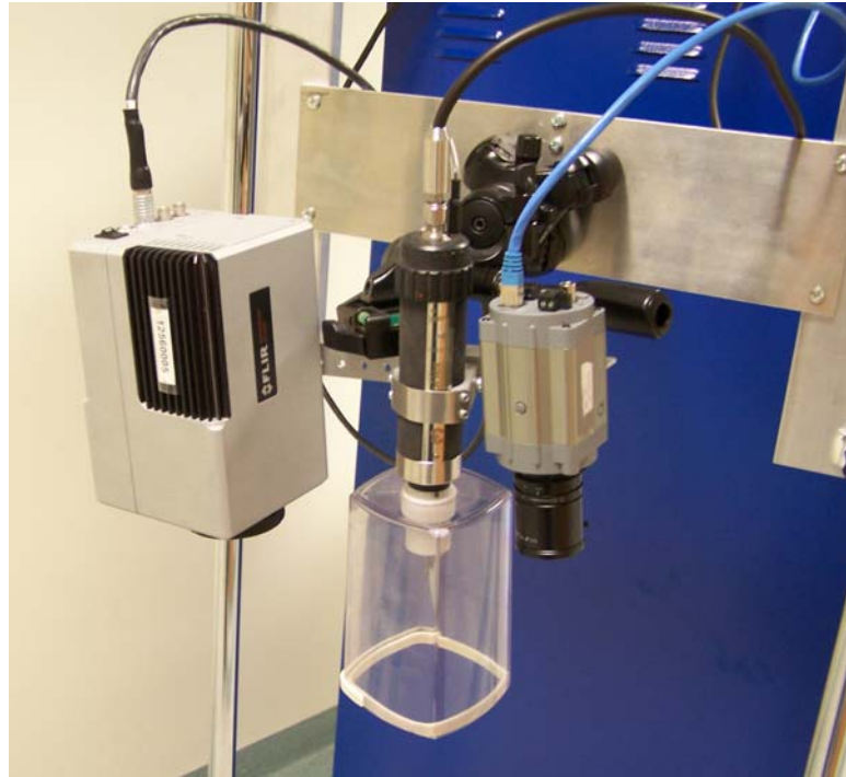
Fig. 3. Basic elements of the diagnostic set – from the left: the high performance cooled quantum well FPA IR-camera, the head of the cryotherapy cooling unit and the RGB camera
