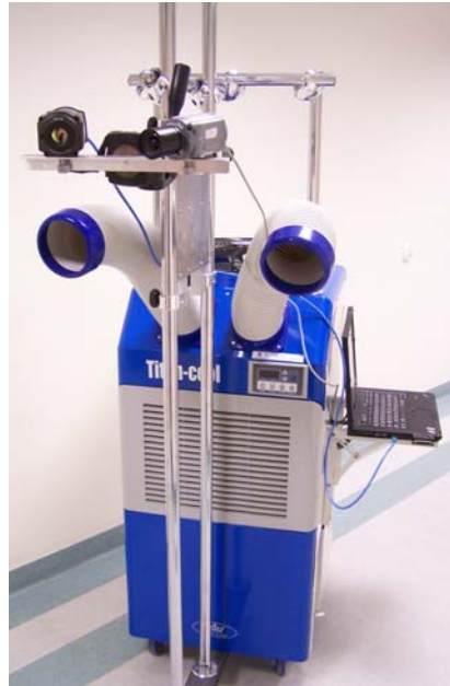
Fig. 5. The diagnostic set with a high power air cooler - IR-camera with room temperature bolometer FPA and RGB camera; two air cooling heads should be directed to the ROI to be cooled; the laptop as the driving-registration unit
