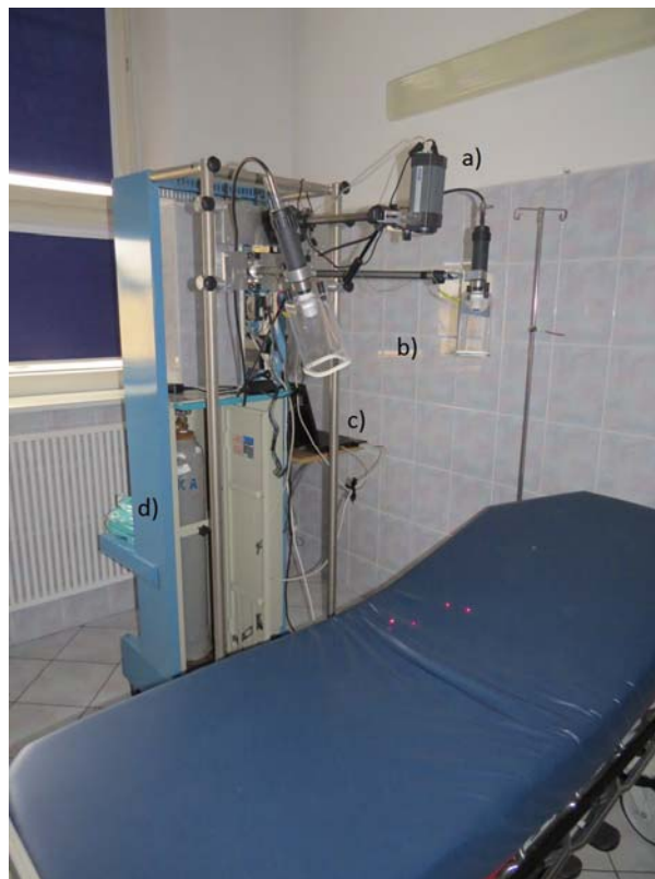
Fig. 4. The diagnostic set in a hospital environment: a) IR-camera with room temperature bolometer FPA; b) two cooling CO 2 heads – red dots on the patient bed show the ROI to be cooled; c) a laptop as the driving-registration unit; d) a standard 19" frame to hold all elements of the system
