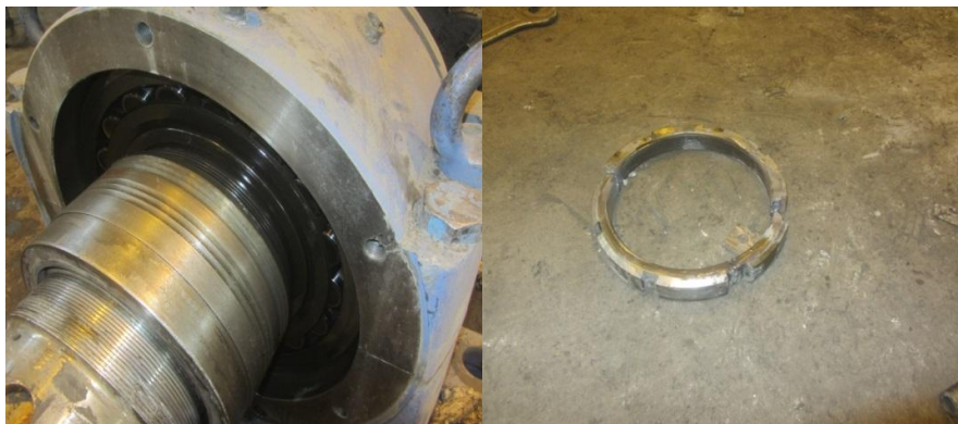
Fig. 8. Crack of chuck nut at bearing point 7
