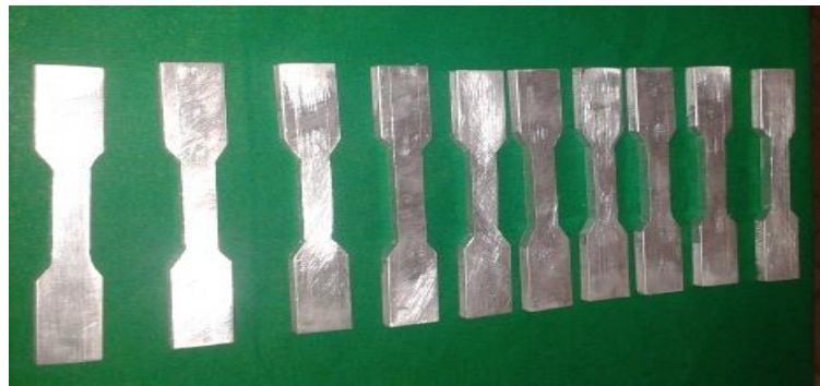
Fig-3 Al/SiC metal matrix composite tensile specimen
