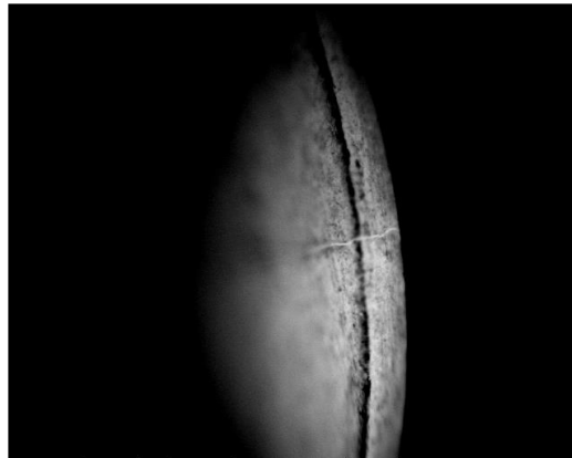
Fig. 8: The best source thermogram of a microcrack made on the side of the valve head
